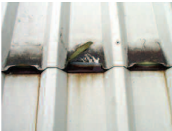
Leathergrain alternative on hot dip galvanised steel substrate roof after 7 years.
