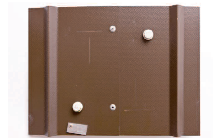
Figure 16. Colorcoat HPS200® with Galvalloy® metallic coating – 6 years exposure at coastal weathering site at Rye, England.
