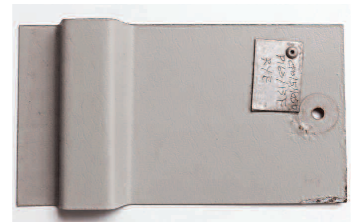
Figure 18. Colorcoat HP200® 18 years exposure at coastal weathering site at Rye, England.
