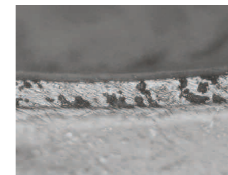
Figure 9. Galvalloy® microstructure after corrosion
