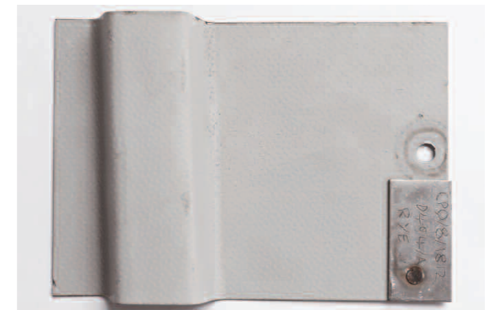
Figure 17. Colorcoat HPS200® with Galvalloy® metallic coating – 13 years exposure at coastal weathering site at Rye, England.
