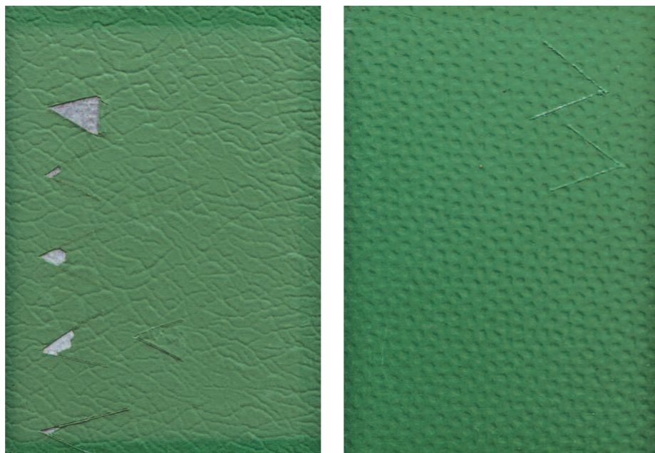
Figure 29. Heritage Green standard leathergrain and Colorcoat HPS200 Ultra® after 2000 total hours in UVB test
