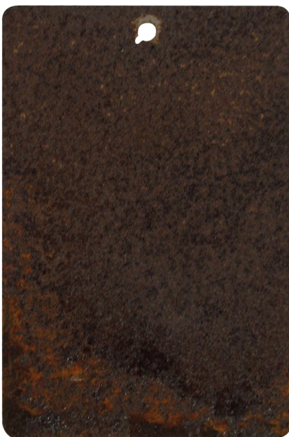
Mild steel corrosion coupon underneath PV panels showing heavy red rust and flaking.
